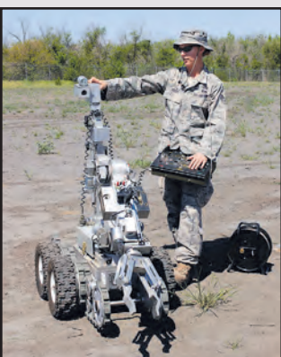
Senior airman Rachel Redel demonstrates how an F6A robot works May 12, 2009 during an explosive ordnance disposal demonstration at Manas Air Base, Kyrgyzstan. The robot is used by the EOD (Explosive Ordinance Disposal) flight for exploration of suspicious items. Airman Redel is assigned to the 377th Mission Support Group at Kirtland Air Force Base, N.M. (U.S. Air Force photo/Tech. Sgt. Elizabeth Weinberg)
