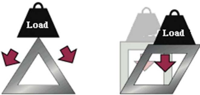
A square will eventually collapse under pressure because the angles can change without having the length of the sides change or bend.
