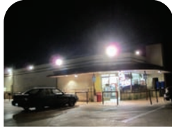
This photo shows an example of glare. The bright spotlights on the top of this building shine right into the eyes of people outside.
