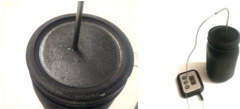
7. Place the wooden block in the bottom of the oven bag. Fill the Mason jar with 500 mL of water. Screw on the cap and insert the thermometer. Put Mason jar in the bag and gather the opening around the probe wire. Tie closed.
