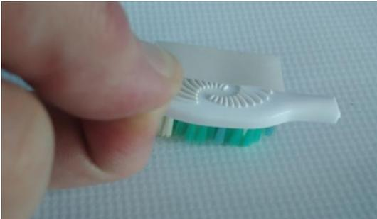
3. Place the motor on one end of the brush on top of the tape. Push down lightly. The motor should still be able to be removed, but it should be able to stay in place during shaking. Hold the motor down further by wrapping the motor to the toothbrush with a rubber band.
