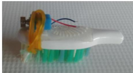
4. Take one end of the motor's wire and place it on the foam. Place the positive (+) side of the battery on the wire and stick to the foam. Touch the other end of the motor's wire to the battery to make sure the motor spins. If it doesn't reverse the wires.
