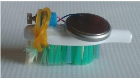
5. When you are ready to activate the Bouncy Bot, place the other wire on the battery and hold in place with second rubber band.
