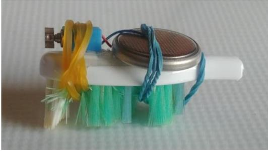
6. If using a AAA battery, place the battery on the sticky foam. Make secure with a rubber band. Place one wire from the motor on one side of the AAA battery. Place the other wire from the motor on the other side of the battery and hold in place with a third rubber band.
