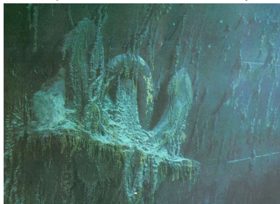
Titanic's anchor weighs over seven tons. Hanging down around and over it are “rusticles” — icicle-like secretions — the waste product of deep-sea bacteria that eat iron in the steel: Courtesy NOAA
