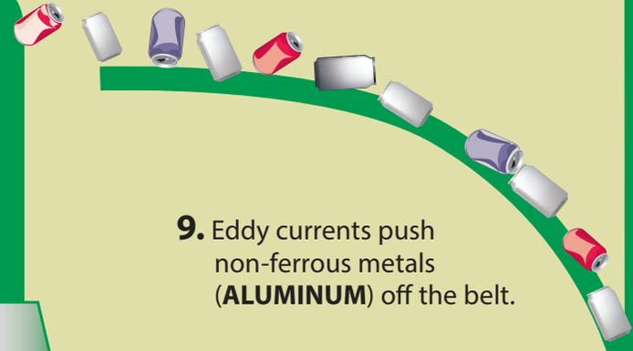
9. Eddy currents push non-ferrous metals (**ALUMINUM**) off the belt.
